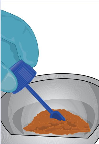
Fig 2a. Wearing gloved hands, use the integral spoon to fill the specimen pot to about a quarter full
